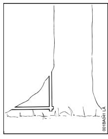
If the tree has large buttress roots, cut into the largest buttress vertically first (horizontally next) and remove the resulting piece.
