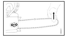
Retensioning during cutting work:
