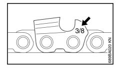
The chain pitch (e.g. 3/8) is marked on the depth gauge side of each cutter.
