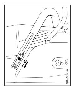
Switching on electric handle heating\*
