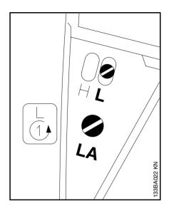
Engine stops while idling: 'L' screw must be one turn open.
