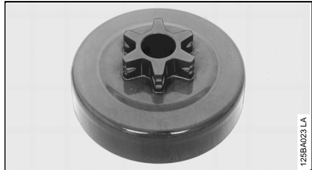
Worn chain sprocket
